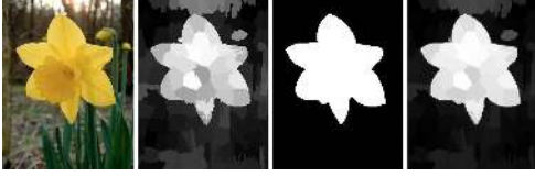
Figure 4. Performance of Graph Cut. Left to right: input, saliency maps without Graph Cut, binary results using Graph Cut, saliency maps after summing up the previous two maps.
