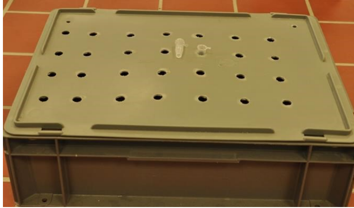
Figure 2. Example of a container with a bored cover to hold Eppendorf-type tubes
