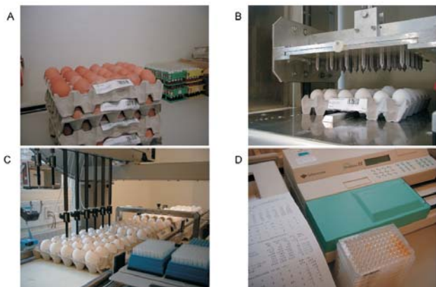
Figure 2. A) Receipt of 60 eggs per producer every 9 weeks (barcode indicating producer is shown). B) The “eggbreaker” punches a hole in 30 eggs at a time. C) Withdrawal of egg yolk from 30 eggs and transfer to microtiter tray. D) Enzyme-linked immunosorbent assay analysis, reading, and transfer of results to central database.
