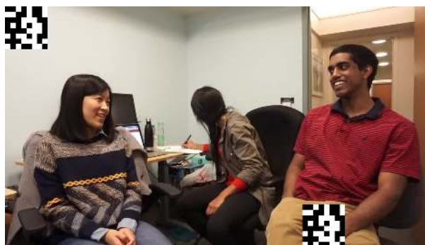
Figure 4: An example barcoded video frame sent by the measurement testbed (§4.2). The barcodes each represent a 64-bit random number that is unique over the course of the video.
