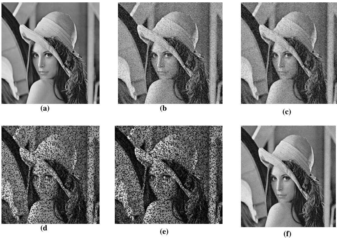
Figure 7. Restoration of Lena image. (a) Original image, (b) Corrupted image with Salt & pepper noise (16.1023 dB), (c) Image recovered by AMF technique (24.4312 dB), (d) Image recovered by GMF technique (11.1253 dB), (e) Image recovered by HMF Technique (10.9820 dB), (f) Image recovered by TSAMFT (t = 60) (34.8523dB)
