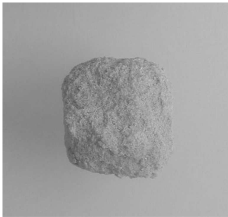
Figure 3a. Sample of FL after 15 cycles: homogeneous behaviour.
