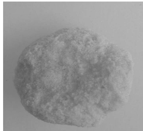
Figure 3b. Sample of SF after 15 cycles: heterogeneous behaviour.
