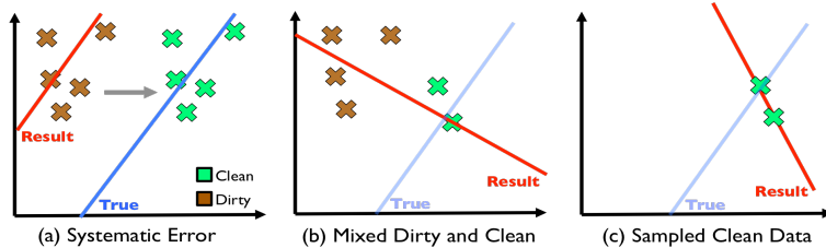
Figure 4: (a) Systematic corruption in one variable can lead to a shifted model. (b) Mixed dirty and clean data results in a less accurate model than no cleaning. (c) Small samples of only clean data can result in similarly inaccurate models.
