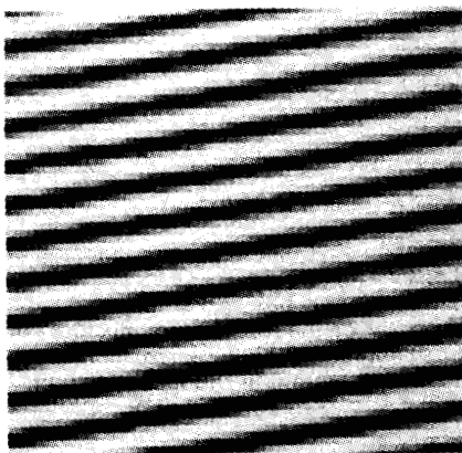
Fig. 20. Sampled-grating moire pattern.
