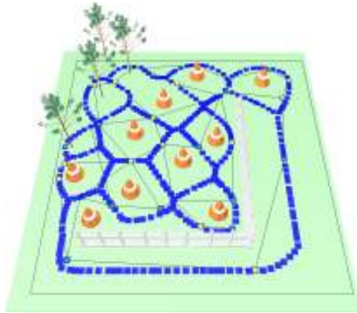
Figure 7.8 Retraction of the roadmap. For each edge in the graph, the local path that corresponds to the edge lies on the medial axis.
