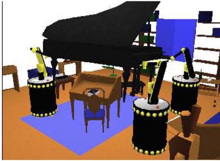
Fig. 1. A “closed-chain” version of the piano mover’s problem. The piano is moved by three cooperating mobile manipulators, creating multiple closed kinematic chains.
