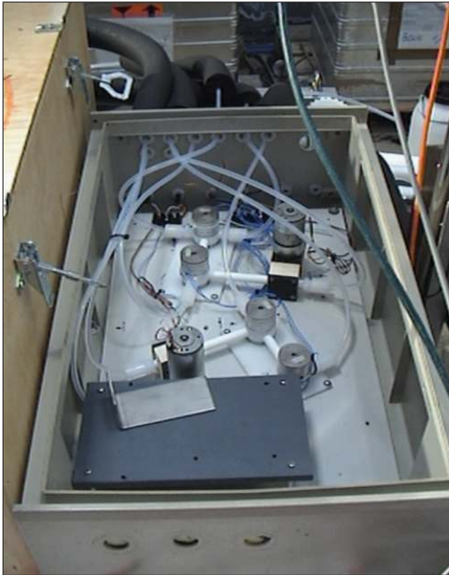
Figure 1. The SESAMO water sampling and distribution system: pumps and valves.
