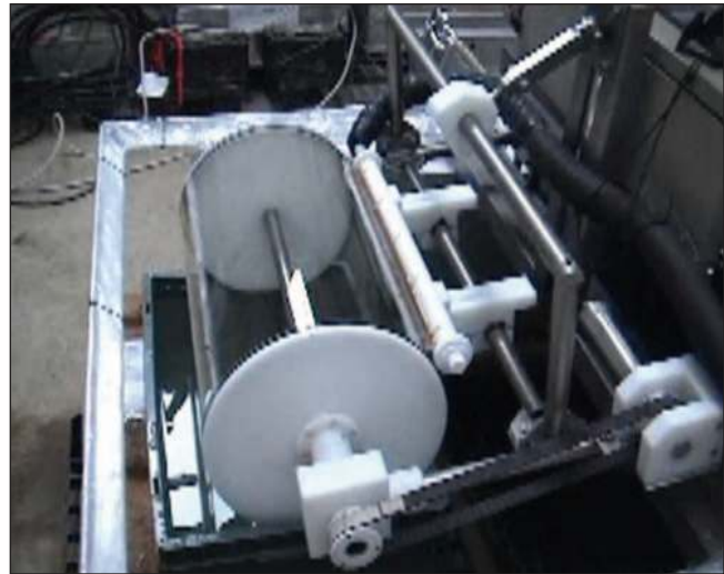
Figure 2. The SESAMO microlayer sampler during in-lab calibration.
