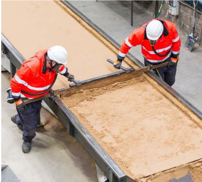
Figure 1: Sand bed being levelled using a strickle
