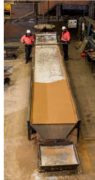
Figure 2: Setup for traditional sand casting of sheet lead
