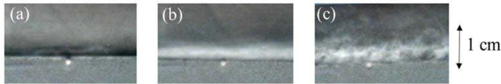
Figure 1.3. Snapshots of sheet flow transport in a small-scale oscillating flow tunnel with fine sand. (a) Start of flow cycle with bed at rest; (b) At maximum orbital velocity, showing a well-developed sheet flow layer with high sediment concentrations; (c) Around flow reversal, showing break-up of the sheet flow layer and the formation of suspension events. Snapshots are taken from video recordings by the author during experiments at the University of Twente as part of the CCM+ development (Chapter 5).
