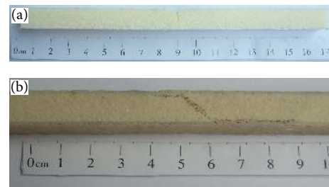
FIGURE 6: Examples of panels produced after conducting flexural strength test of composites reinforced with (a) fabric and (b) mat.
