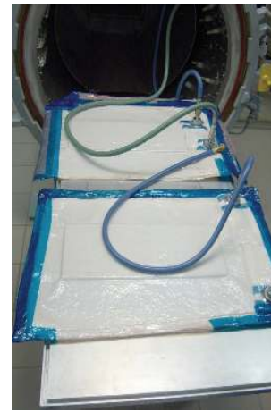
FIGURE 1: Vacuum packages before transport to autoclave.
