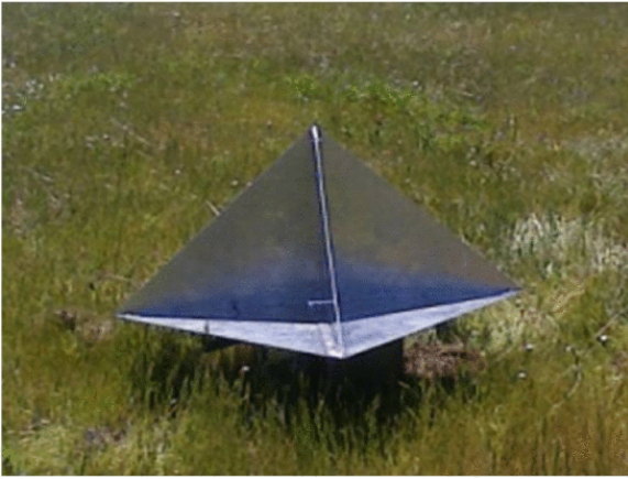
Fig. 15. Experiment I: Vibrating Target on the Test Ground near Julian, CA. the Target is an Aluminum Triangular Trihedral with a Lateral Length of 21 in. the Vibration Frequency and Amplitude were 1.0 Hz and 1.5 cm, Respectively.
