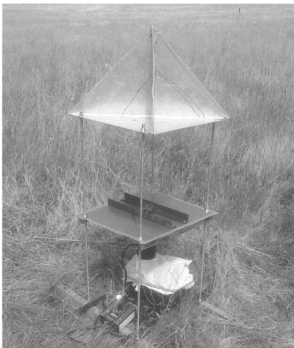
Fig. 20. Experiment II: Vibrating Target on the Test Ground Near Julian, CA. the Target is an Aluminum Triangular Trihedral with a Lateral Length of 15 in. the Actual Vibration Frequency and Amplitude were 5.0 Hz and 1.5 mm, Respectively.
