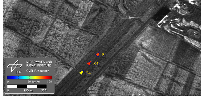
Fig. 8. SAR image acquired with DLR’s new X-band four-channel F-SAR system containing three detected moving targets. Detection was done using the proposed algorithm (horizontal axis: range; vertical axis: azimuth).
