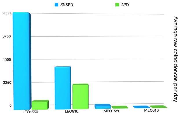
Fig. 6 Average raw coincidences per day as reported in Table 3. Shown are results for a LEO with inclination 50 degrees and height 600 km and a MEO with inclination 60 degrees and height 8000 km, and for wavelengths of 810 and 1550 nm with avalanche photo detectors (Si-APD @ 810 nm, InGaAs-APD @ 1550 nm; green bars) and super-conducting nanowire single photon detectors (blue bars).
