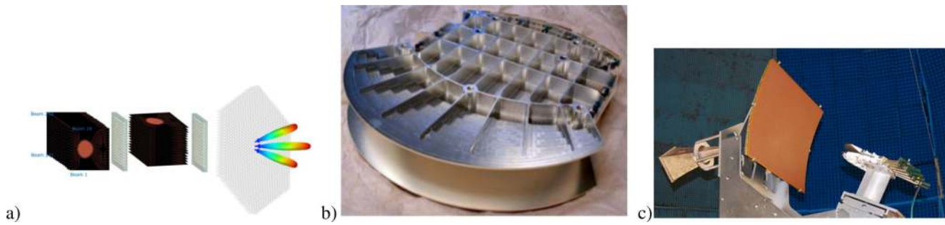
Fig. 11. a) Double layers of Rotman lenses producing pencil beams in two directions; b) Continuous parallel plate waveguide lens-like antenna; c) Prototype of a QOBF antenna [89].
