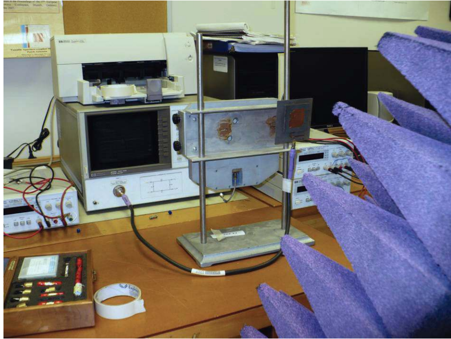
Fig. 5.2 Measurement setup of S11
