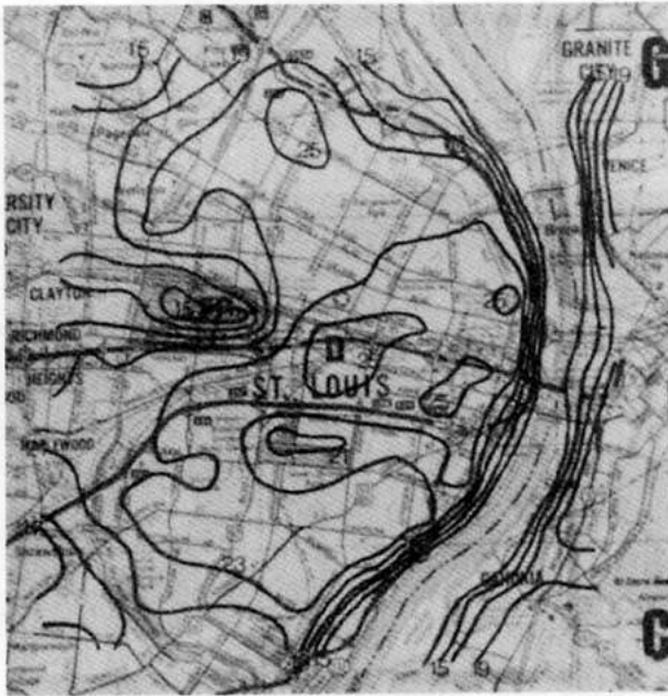
FIG. 17. Enlargement of unsmoothed surface heat flux ( W\ m^{-2} \times 0.1 ) over downtown St. Louis at approximately 1330 LST 10 June 1978.
