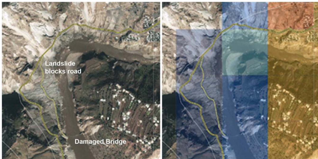
Fig. 4. Damage assessment for the northern Muzaffarabad city area, Muzaffarabad District, Pakistan (1 : 7500). Visual interpretation on pre- and postdisaster images with 250 \times 250 m grid cells is applied to interpret damage to infrastructure and build-up areas by means of UN housing damage classification: no damage, moderately damage ( < 33\% ), severely damage ( 33\%–66\% ), and completely destroyed ( > 66\% ). Semitransparent color map overlay is used to visualize damages, and blue-colored grid cells show those areas with moderate (light blue) to high (dark blue) damage to infrastructure, whereas the orange- and red-colored grid cells show damage to build-up areas.
