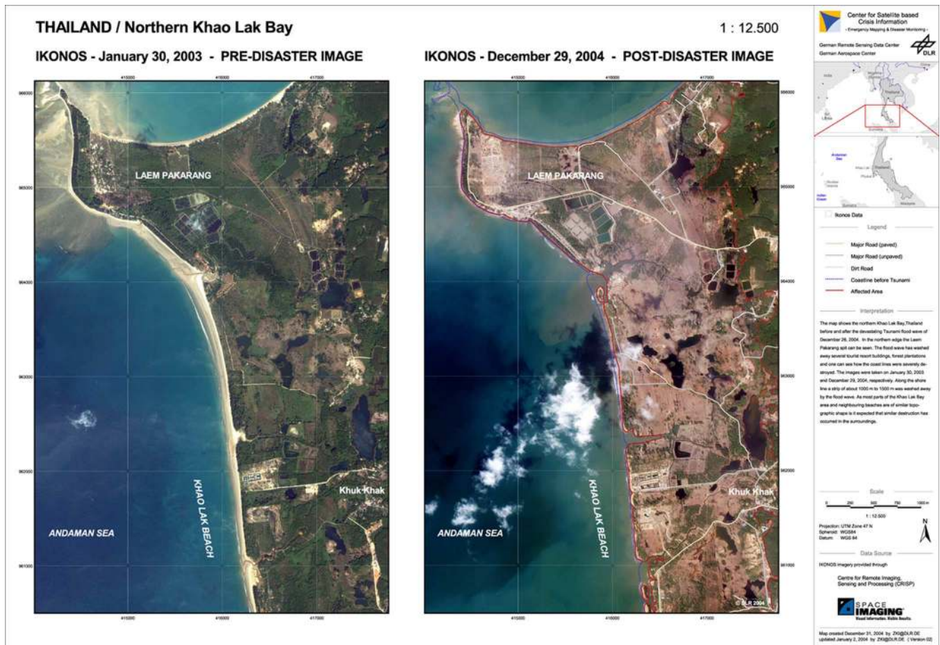
Fig. 2. High-resolution satellite map from new and archived satellite imagery of the northern Khao Lak Region, Thailand (1 : 12.500). The archived pre-disaster and new acquired postdisaster satellite images allow easy and quantitative damage assessment by visual change detection. Tsunami-affected areas are delineated using a red polygon signature, and in blue, the coastline before the tsunami is indicated.
