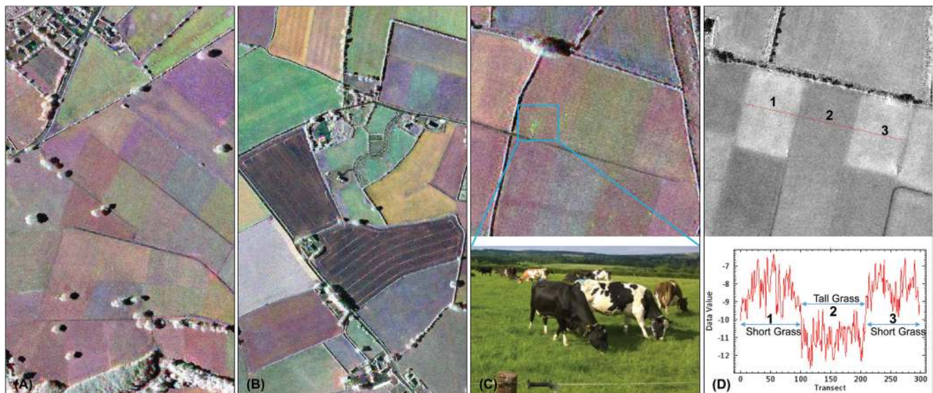
Figure 3: TerraSAR-X Staring Spotlight colour composite (R: 08-06-2014, G: 19-06-2014, B: 11-07-2014) of Teagasc Curtin Farm. Potential of very high-resolution microwave radar (TerraSAR-X) data: (A) Monitoring of hedges and individual tree count, (B) furrow/plough lanes, (C) possibility to detect the location of grazing herds if they are standing close to each other and (D) inter and intra paddock variation.
