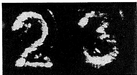
Fig. 4. Photograph of the diffracted phase-conjugate image carried by beam 3.
