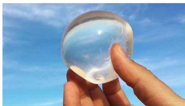
Fig. 10 An edible and biodegradable pouch made of seaweeds as a handy container for fresh water. https://shorturl.at/bjEJQ
