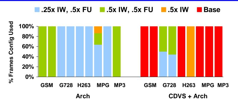
Most energy efficient architecture depends on presence of DVS
