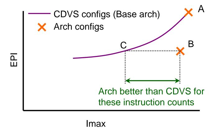
For G728, EPI of adapted architecture < Base for base frequency
