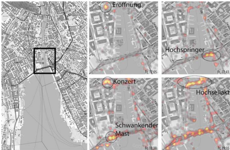
Fig. 6 Pedestrian densities during the Zürichfascht festival for multiple attractions (the opening ceremony, a high diving competition, a concert, a high wire performance) at different times and locations
