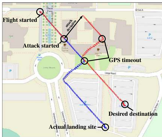
Fig. 9: The actual GPS data gathered from the sensor data (blue) is tampered with by the attacker before being sent to the autopilot. The autopilot then receives a corrupted set of GPS coordinates (red) and makes the “necessary” adjustments in order to return to the established path. The autopilot thinks that the drone reached the desired location, but it has actually deviated.
