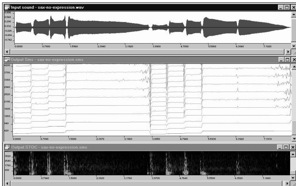
Figure 1: Snapshot of SMS analysis and synthesis graphical interface for the beginning of the ‘Autumn Leaves’ theme. The top window shows a graphical representation of the input sound file, the middle window shows the evolution of the partials’ frequency, and the bottom window shows the spectral residual.
