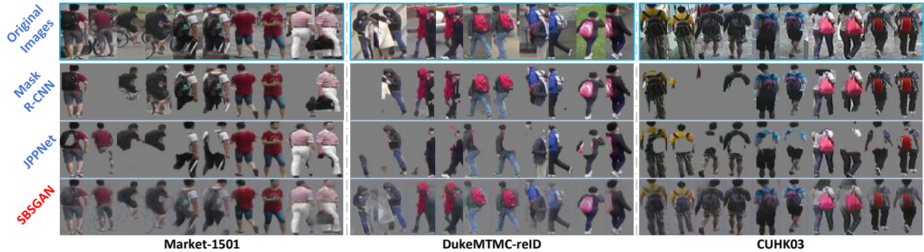
Figure 4. Comparison between hard-mask and soft-mask images. Images are selected from three different person re-ID datasets. The original images are listed in the first row. The second and the third rows respectively show hard-mask images by Mask-RCNN [1, 13] and JPPNet [25]. The last row shows our soft-mask images generated by the proposed SBSGAN.
