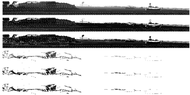
Figure 4. A range image example. It is cropped to only show the front 90^\circ . The first three rows are range, intensity, and elongation from the first LiDAR return. The last three are range, intensity, and elongation from the second LiDAR return.
