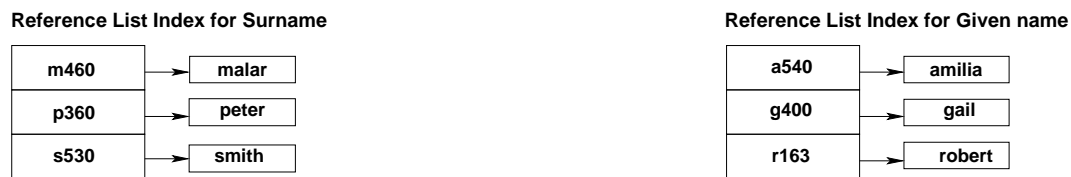
Figure 8.7: The Reference List Index (RLI) for Surname blocks and Given name blocks. In the example, we use one reference value per block. RLI is generated in step 4 of the protocol.
