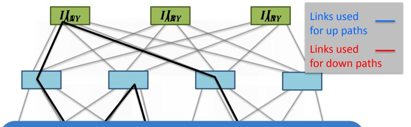
[ IP anycast + flow-based ECMP ]
