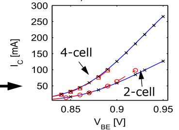
Excellent match for coupled thermal network (crosses) and *derived* lumped thermal resistance (solid line) for 2-cell and 4-cell transistor
