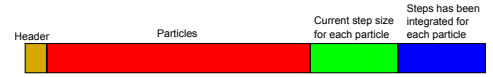
Fig. 5: An example that shows the structure of a seeding curve segment. The yellow header includes three floating point numbers representing the number of steps this seeding curve segment has advanced, the ID of the original seeding curve it comes from, and the number of particles on the seeding curve. The red part is the particles. The green part is the current step size for each particle and the blue part is the number of steps that have been integrated for each particle.
