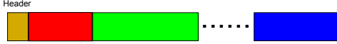
Fig. 7: An example that shows the structure of the message containing the tasks stolen by the thief. Suppose the thief stole N seeding curve segments. The yellow part is the header that includes N + 1 floating point numbers. The first number represents the number of the seeding curve segments. The following N numbers are the length of each seeding curve segment. The remainder is the N seeding curve segments.
