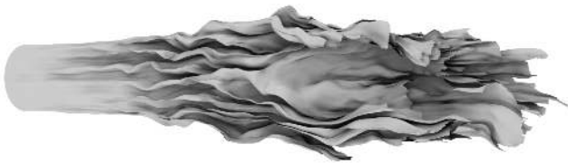
Figure 4: A stream surface in the thermal hydraulics dataset illustrates the strong turbulence in flow leaving an inlet.
