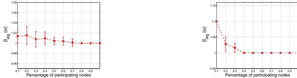
Fig. 3. cDSMA accuracy for 10x10 nodes B-A graphs(left) and grids(right) as a function of the 1-median subgraph size: uniform service demand distribution.
