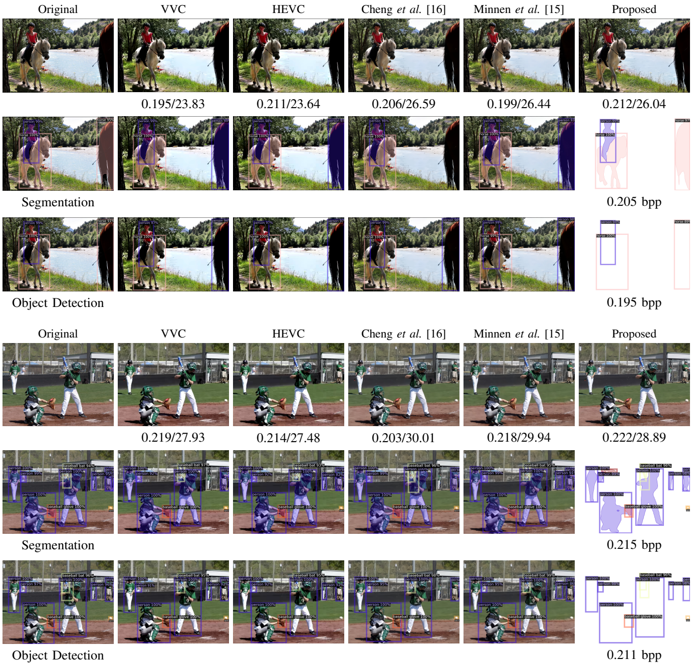
Fig. 16. Illustration of object detection, segmentation, and input reconstruction results for several benchmark methods and our 3-layer network on two images: the top three rows correspond to the first image, and the bottom three rows to the second image. For each input image, the top row shows input reconstruction, the next row shows object segmentation, and the last row shows object detection. The first column shows the original images and the results of object detection and segmentation produced by the FPN-based R-CNNs applied to those images. The detection and segmentation results are overlaid on the original images. The next four columns show the images encoded and decoded by various benchmarks, and the FPN-based R-CNN results produced from decoded images, again overlaid on those images. Two numbers are shown beneath each image, indicating the bitrate and RGB PSNR, respectively, in the format bpp/PSNR(dB). The last column shows the outputs of our 3-layer network. Object detection and segmentation results are shown on a blank background, because our system does not need to reconstruct the input image in order to perform object detection or segmentation. For these cases, only the bitrate is shown beneath each result. To reduce the clutter, in all cases we only show objects with a confidence score of over 80%.
