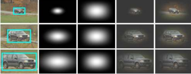
Figure 1. Gaussian and cosine window filtering raw pixel value example. The tracked region has a size of (175 \times 113) . First column: same regions with targets at three different scales (i.e., small (56 \times 32) , medium (110 \times 61) , large (164 \times 83) ). Second column: Gaussian windows according the target size (i.e., small (\sigma_w = .32, \sigma_h = .28) , medium (\sigma_w = .63, \sigma_h = .54) , large (\sigma_w = .94, \sigma_h = .73) ). Third column: cosine window for all the three examples (i.e., size (175 \times 113) ). Fourth and fifth columns: images filtered with Gaussian and cosine windows respectively. Figure shows how the fixed cosine window fails to represent the target compared to the Gaussian windows. The cosine window includes background for small targets and discards information for big targets.
