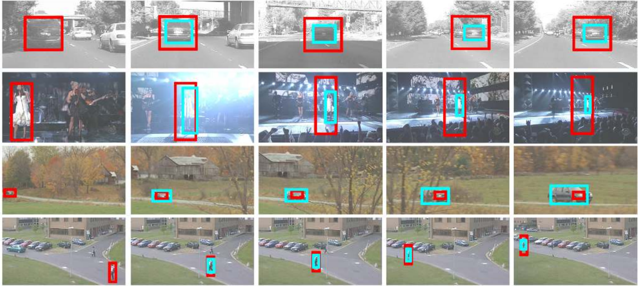
Figure 3. Some sequence examples with scale changes and the responses from KCF (i.e., red boxes) and sKCF (i.e., light blue boxes). The first column represents the initial selection and the size of the tracker at the first frame in the sequence.
