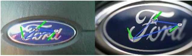
Figure 5: Two triangles that match across images. Green lines show the orientations of the features. The numbers denote the visual word label.
