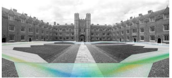
Fig. 1. Illustration of a magnetic field map built using our SLAM approach. Each hexagonal block (with radius of 5 m and height of 4 m) covers a Gaussian process magnetic map volume of \sim 260 \text{ m}^3 in a state dimension of 256. A more detailed map is provided in Fig. 5.
