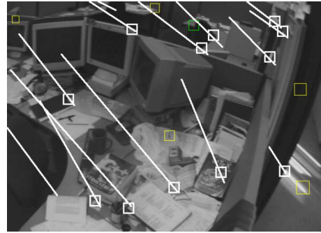
Figure 8. New landmarks being observed in the image. Epipolar lines, according to the mode particle's estimate, are overlaid. The distance of observed landmarks from their epipolar lines can help constrain pose: See Figure 9.
