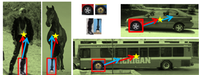
Figure 1. Features of different object classes can share appearance although they do not necessarily also share their location. For instance, the legs of a person and a horse share both appearance ( bounding boxes ) and location ( arrows ) whereas the wheels of a bus and car are similar in appearance but not in location ( red/blue arrows ). In this paper, we are building a multi-class detection algorithm by using discriminative features.
