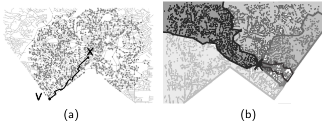
Figure 1: (a) A map of Silver Spring, MD, and the vertices, highlighted by circles, that are visited by Dijkstra’s algorithm in determining the shortest path from X to V , and (b) its partition into regions r_i such that the shortest path from X to a vertex in r_i passes through the same vertex among the six vertices that are adjacent to X (i.e., the shortest-path map of X ).
