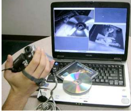
Figure 10. A snapshot of the CD-cover recognition running. With 40000 images in the database, the retrieval is still real-time and robust to occlusion, specularities, viewpoint, rotation and scale changes. The camera is directly connected to the laptop via firewire. The captured frames are shown on the top left, and the top of the query is displayed on the bottom right. Some of the CD-covers are also connected to music that is played upon successful recognition.
