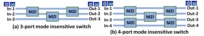
Fig. 2. Schematic of the proposed mode insensitive switch matrices; (a) 3 \times 3 switch; (b) 4 \times 4 switch.
