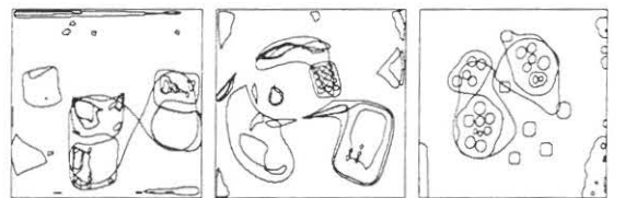
Figure 9: Blob boundaries of the 50 most significant dark blobs in (a) the toy block image (b) the telephone and calculator image and (c) the dot pattern image.
