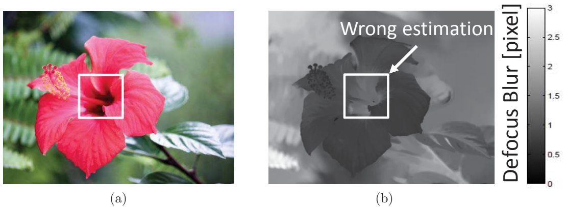
FIGURE 2.9: Illustration of the blur texture ambiguity, adapted from [6]. (a) is the input image and (b) is the full defocus map. In the white boxed region, a wrong defocus estimation occurred due to the texture of the flower.
