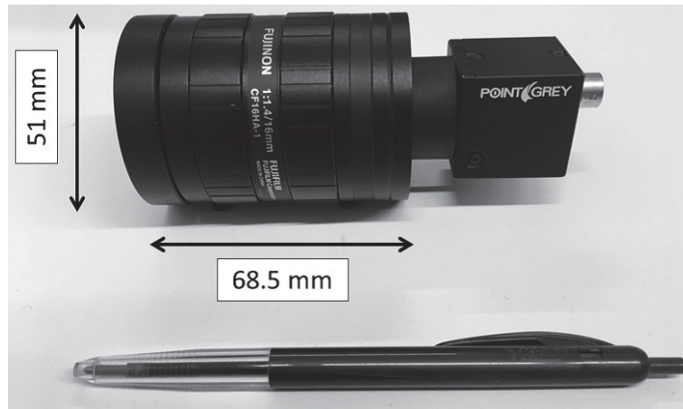
FIGURE 4.5: The camera and lens used in Experiment 1. The field of view is about 37-degree width.
