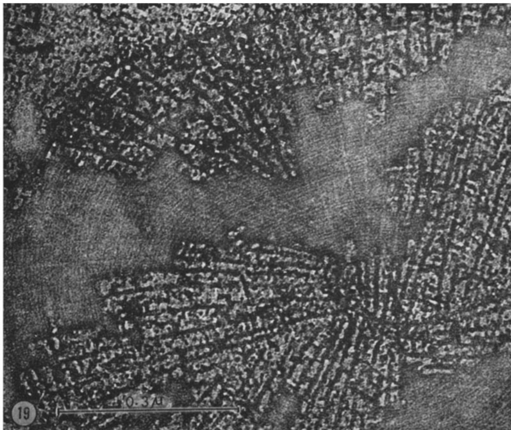
FIGURE 19 Higher magnification of a scale similar to those shown in Fig. 18, demonstrating the frequent, oriented array of the covering pectic mass in organized tiers in between the radial microfibrils. Negatively stained with 2% PTA, pH 7.2. \times 160,000 .
