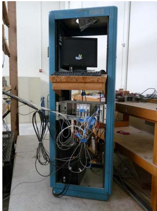
Figure 4.2 – Signal conditioning and data acquisition module with instrumentation wiring
