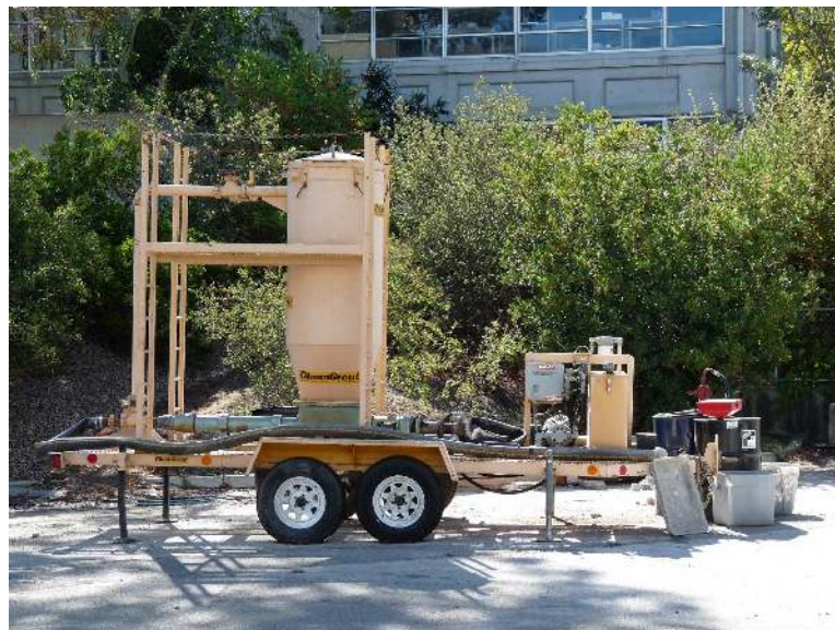
Figure 4.7 - ChemGrout mixer used to mix model soil
