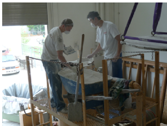
Figure A.4 – Mixing dry material in a wheel barrow and adding it to the tank
