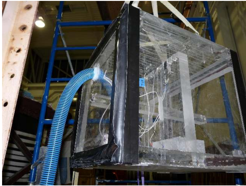
Figure 4.15 - Fully assembled model structure with soil barriers and flexible tubing to accommodate instrumentation wiring
