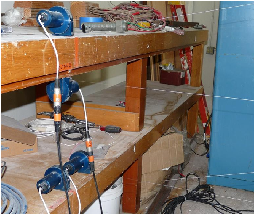
Figure 4.4 - Four wire potentiometers mounted off of shake table
