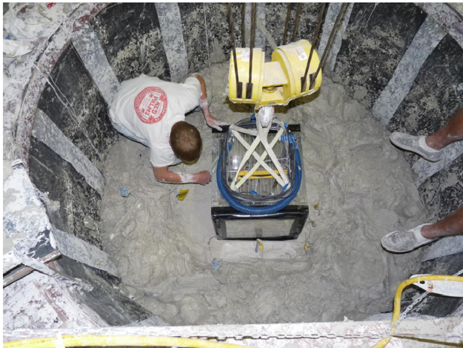
Figure 4.17 - Positioning of subway model in testing container using the overhead crane (shaking direction in photograph is approximately left to right)
