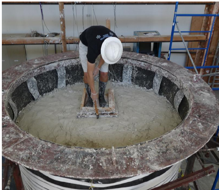
Figure 4.14 - Top-down hammer blow testing using a framing hammer
