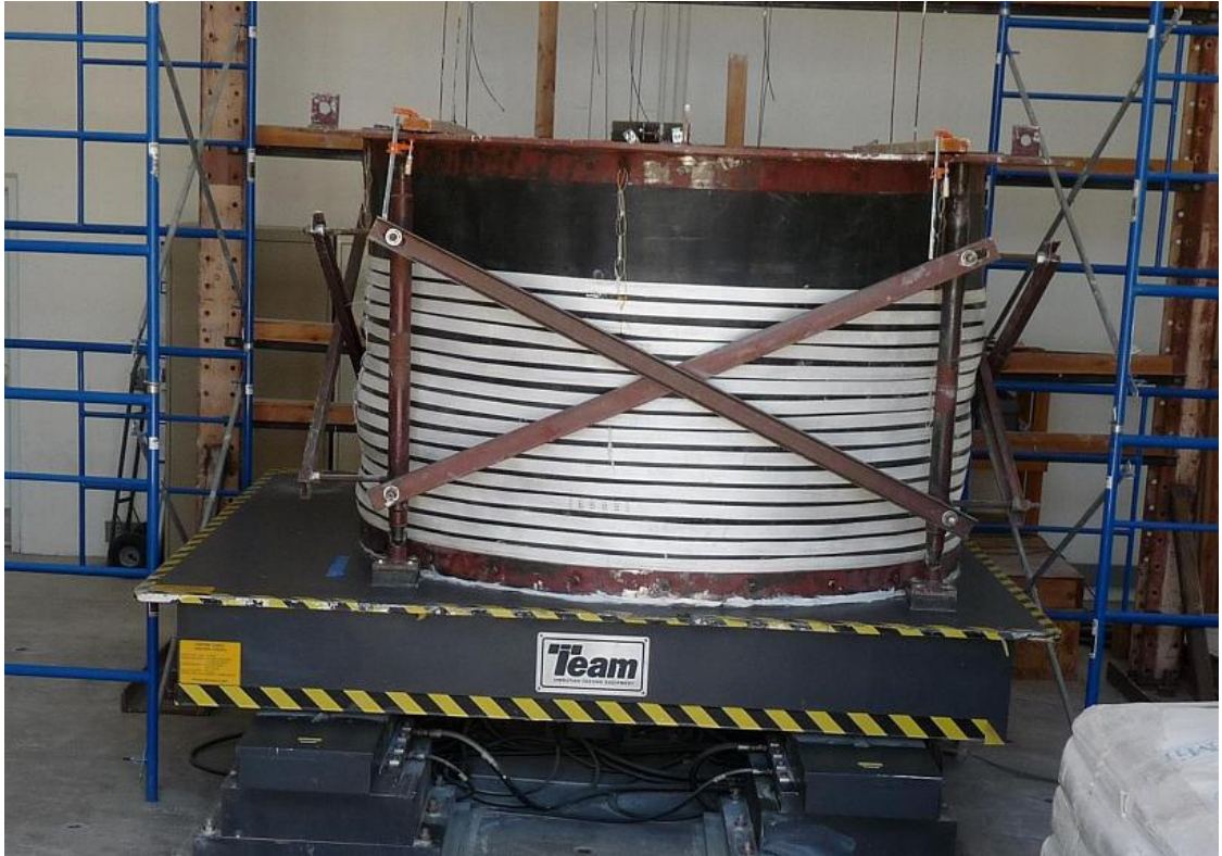
Figure 3.10 - Fully assembled testing container mounted to the shake table (the cross-braces are removed during testing)
