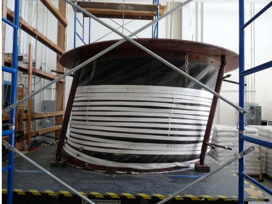
Figure 4.13 - Deformed Phase I free-field model before soil reconstitution
