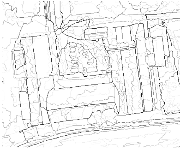
Figure 2: The contour disappearance map associated with the scale-sets of figure 1 (logarithmic scale).
